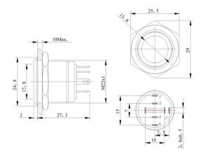
the direction of the arrow is the LED common pin 1,2,3,4 are LED positive poles other 2 pins are push button
